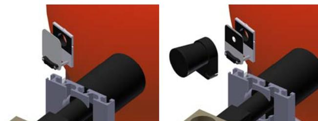
*The quick-change holder on the 8° port enables fast exchange of plugs and light traps*
