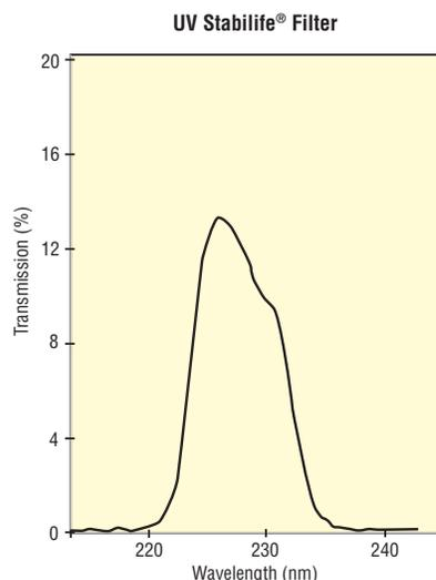
Stabilife UV narrow bandpass filter @ 228nm, fully blocked to 50D
