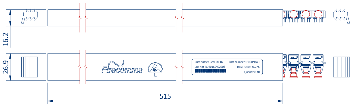
FIGURE 3 Packing tube for Firecomms Horizontal RedLink® Receivers
