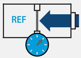
• Absolute pressure references the pressure in a vacuum (0Pa), a measurement used in applications such as altimeters.
