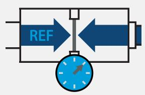
• **Differential pressure** references a different dynamic pressure in the system rather than atmospheric pressure. This method is used to maintain a relative pressure between two vessels such as compressor tanks.
