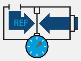
Gauge pressure references the ambient atmospheric pressure to provide a pressure measurement that excludes the effects of atmospheric pressure. This method is used in blood pressure monitors and when measuring tyre pressure.
