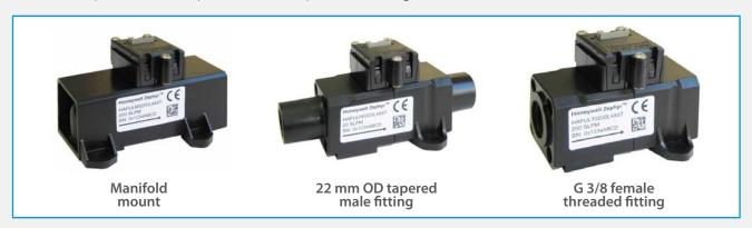
Zephyr<sup>™</sup> SLPM sensors are designed to measure mass flow of air (uni-directional) and other non-corrosive gases. Seven standard flow ranges are available 0-10 SLPM, 15 SLPM, 20 SLPM, 50 SLPM, 100 SLPM, 200 SLPM or 300 SLPM, with custom flow ranges available. The sensors are fully calibrated and temperature compensated (0°C to 50°C) with an onboard Application Specific Integrated Circuit (ASIC) providing a response time of 1 ms.
