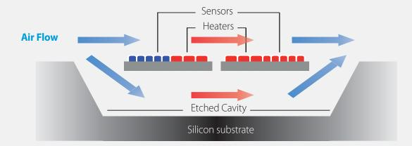
The heater resistor maintains a constant temperature, 160°C above ambient, during sensor operation. Airflow moving past the chip transfers heat from the heater resistor. This airflow warms the downstream resistor and cools the upstream resistor. The temperature change and the resulting change in resistance of the temperature resistors is proportional to the mass airflow across the sensing element.
