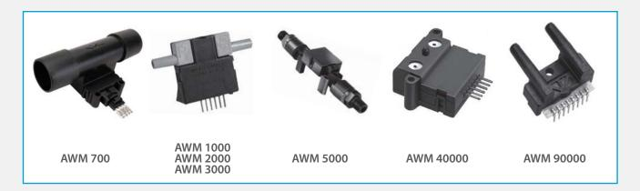
**AWM 700** series mass airflow sensors provide in-line flow measurement with specially designed bypass flow housing. The sensors measure flow as high as 200 SLPM while inducing a pressure drop of 1 inch  $\rm H_2O$ , typically. The AWM700 has a high-flow-range capability in a small package.
